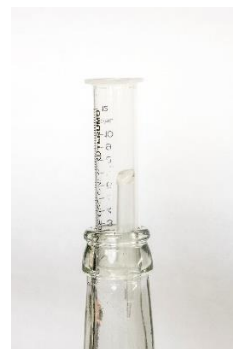
Figure 25 – Two examples of airlocks used for fermentation to allow the escape of fermentation gasses while restricting the diffusing of oxygen back into the system
