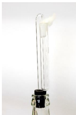
Figure 25 – Two examples of airlocks used for fermentation to allow the escape of fermentation gasses while restricting the diffusing of oxygen back into the system
