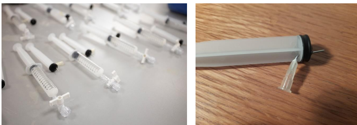
Figure 18 - Syringes and needles repurposed to function as chromatography columns
